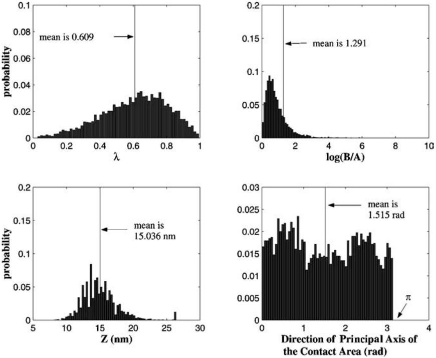
**FIGURE 9** Statistics of the reconstructed glass surface.
