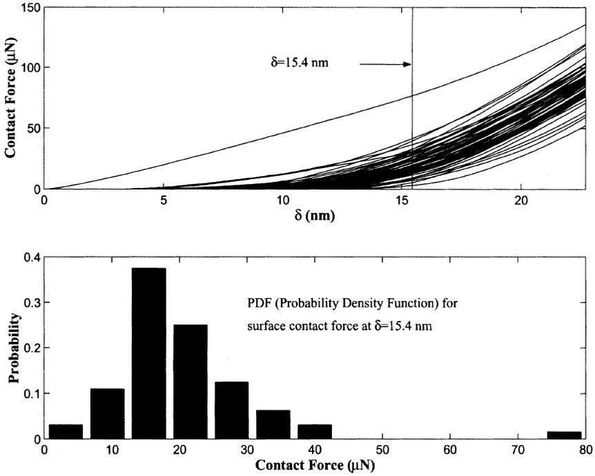
**FIGURE 12** The overall load-displacement relationship at  $\delta = 15.4$  nm.
