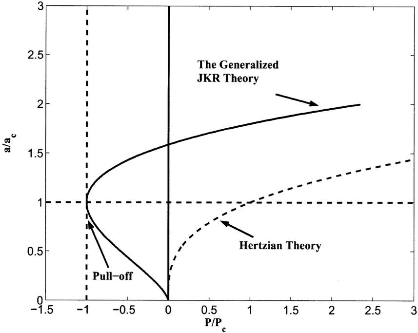
**FIGURE 3**  $a/a_c$  versus  $P/P_c$  for a single asperity.
