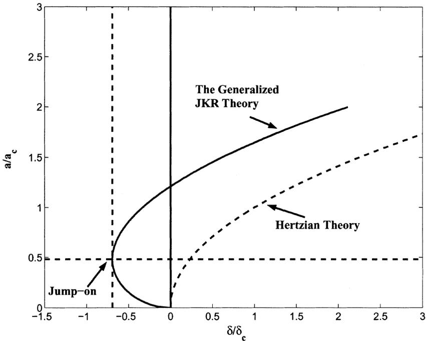
**FIGURE 2**  $a/a_c$  versus  $\delta/\delta_c$  for a single asperity.
