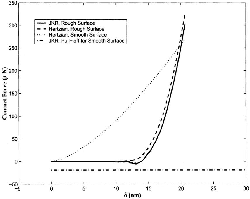
**FIGURE 15** The load-displacement relationship for rough surface contact.
