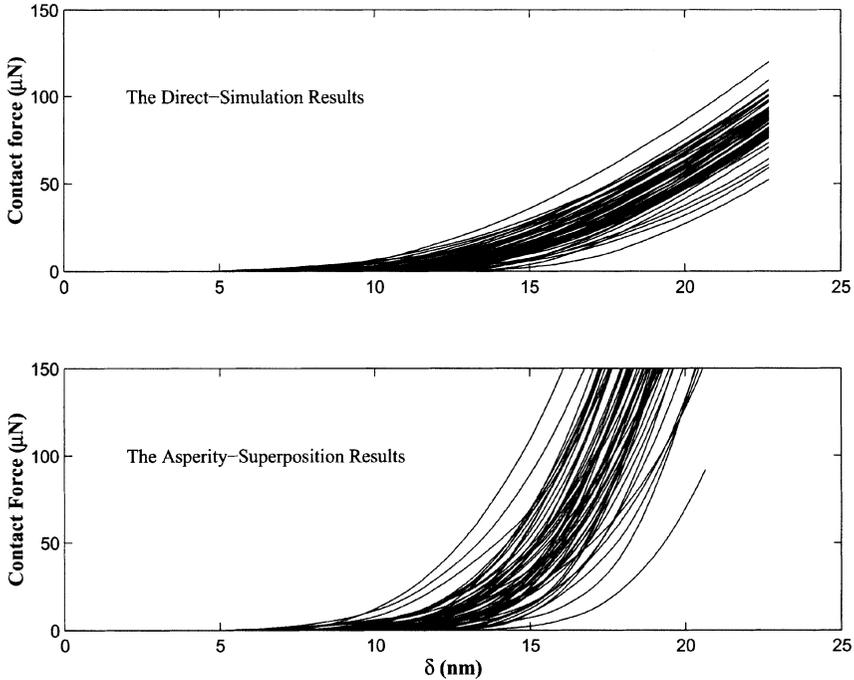
**FIGURE 14** The load-displacement relationship for rough surface contact.
